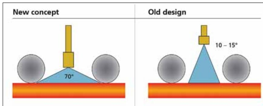
**Figure 6.** The new spray nozzle design can cope with hard cooling practice
