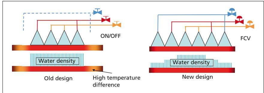
Figure 7. Spray width control to avoid corner cracking
